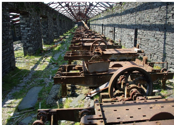
'Australia' Gallery Mill Saw Tables, Dinorwig Slate Quarry (Component Part 2) © Gwynedd Archaeological Trust
