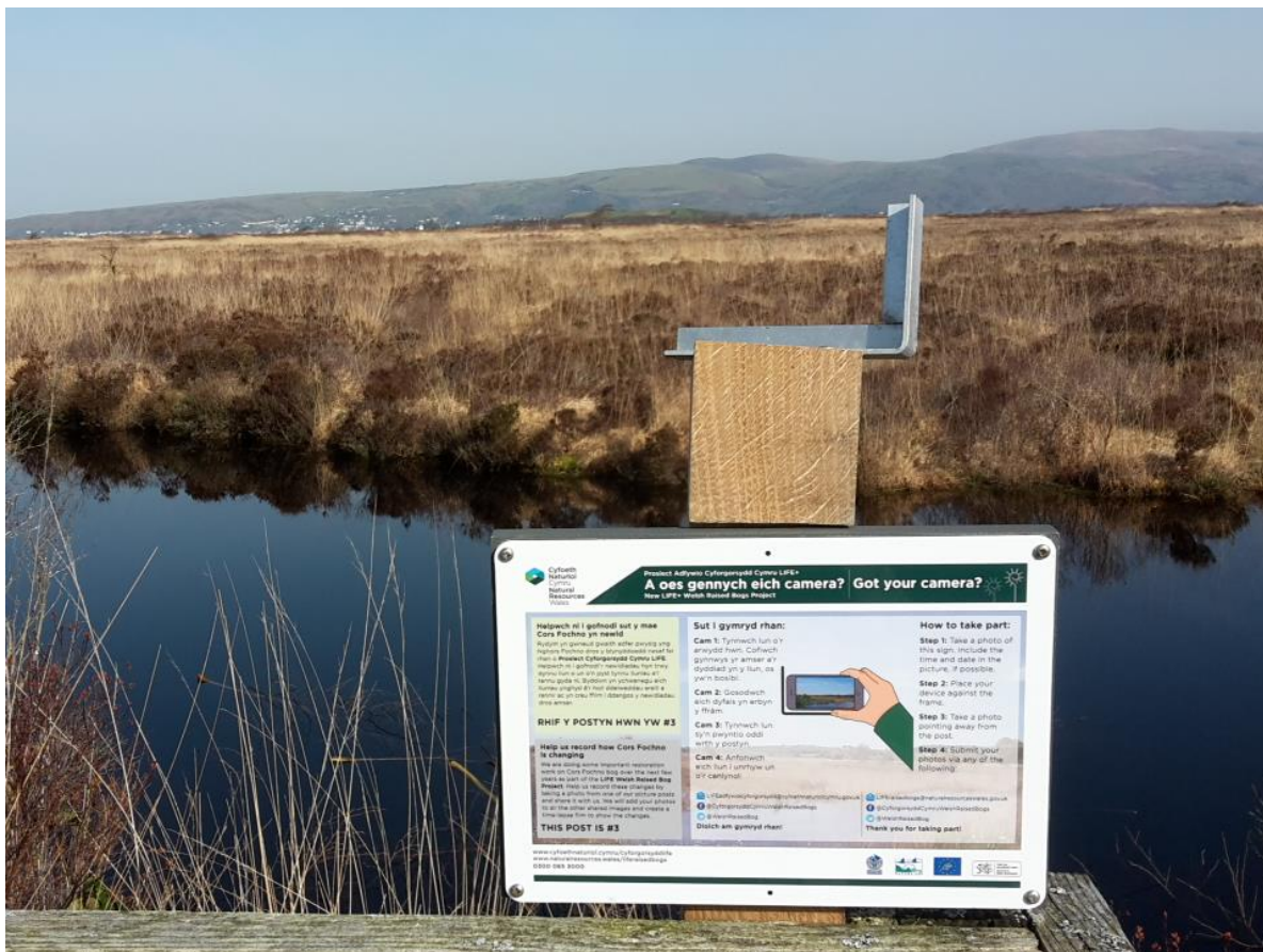
An example of a fixed-point photo bracket installed at Cors Fochno in the Dyfi Valley © Naomi Davies.
